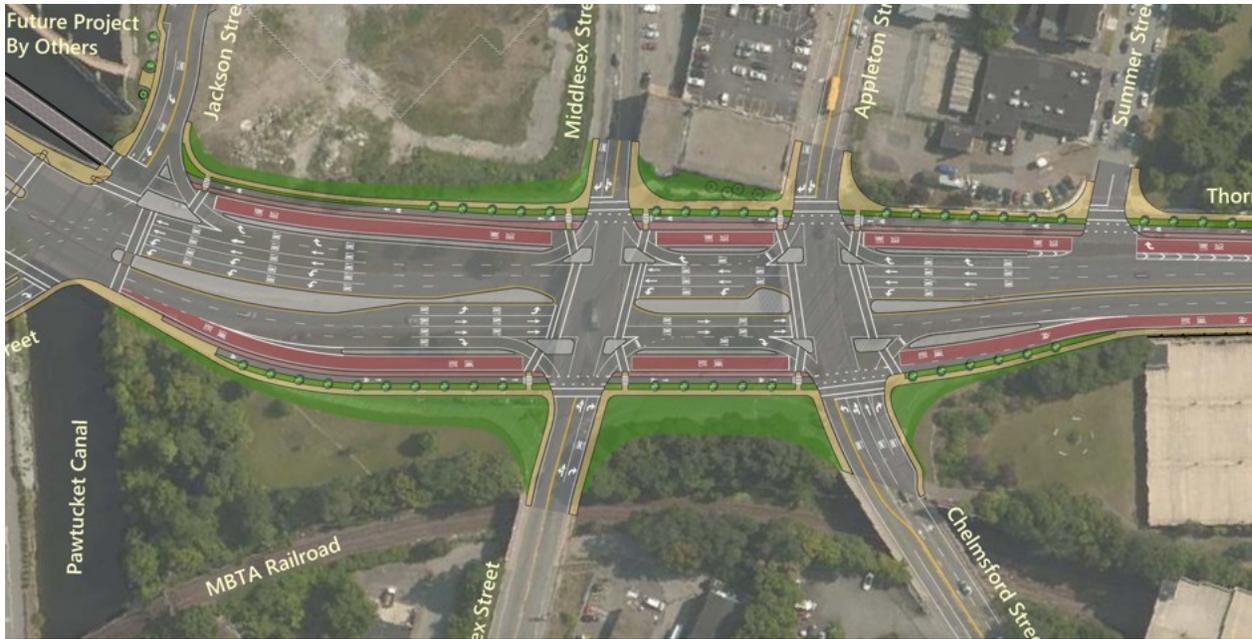
Figure 2: Rendering of the Lord Overpass reconstruction. (Image from article. Courtesy City of Lowell)
