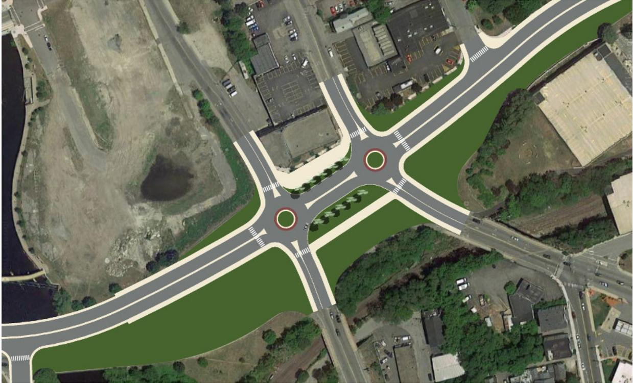
Figure 3: A quick and rough model of what I described above. Some measurements may be a bit off—maybe the roundabouts should be somewhat bigger. The layout of lanes can be changed as desired, but should only include what can fit along the rest of the street beyond these two junctions.
