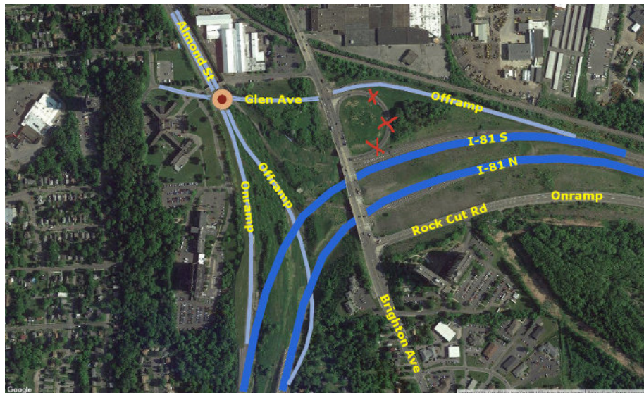
Figure 36: I-81S junction at Almond St (Full Street-grid plan): A roundabout replaces the proposed diamond junction at Glen Ave.
