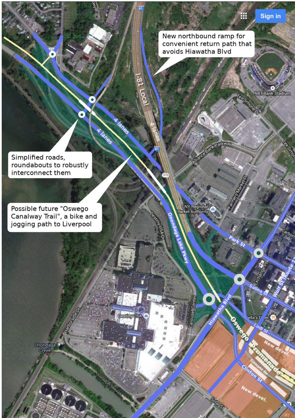
Figure 7: A redesign of the confluence of Onondaga Lake Pkwy, Park St, and I-81: simplified roadways; improved inter-connectivity; the I-81S Exit 23 flyover ramp is kept; and a new return path to I-81N is created that avoids using Hiawatha Blvd, greatly reducing traffic load on that street. A single roundabout option at OLP/Park St/I-81 double roundabout should also be analyzed.
