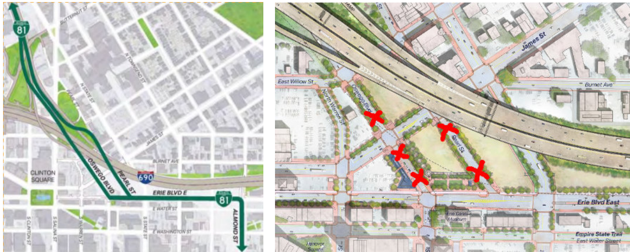
Figure 23: Proposed NYSDOT Canal District: Not realistic as planned; Oswego St and Pearl St become highway on/off ramp roads that cut through the center of the District, undermine a new park, and additionally burden Erie Blvd (“Erie Way”)—the would-be main drag of the District.
