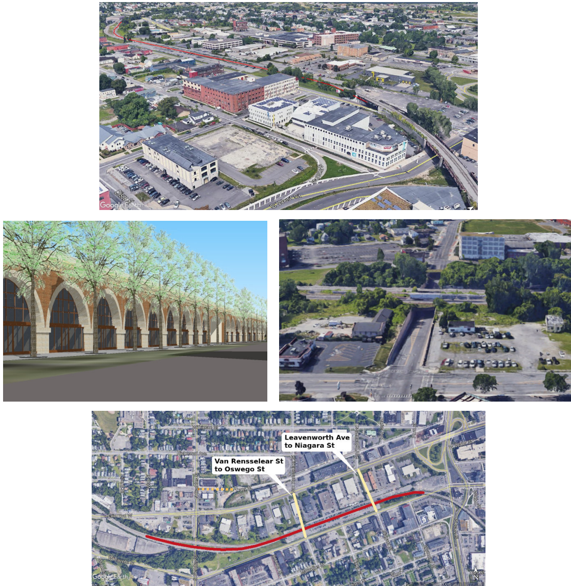
Figure 30: Elevated railroad along W Fayette St: removes a multi-block barrier between W Fayette St and “Erie Way”; archway viaduct (left); eliminates pedestrian-dangerous Geddes St railroad underpass (right); allows useful street-grid connections (below).
