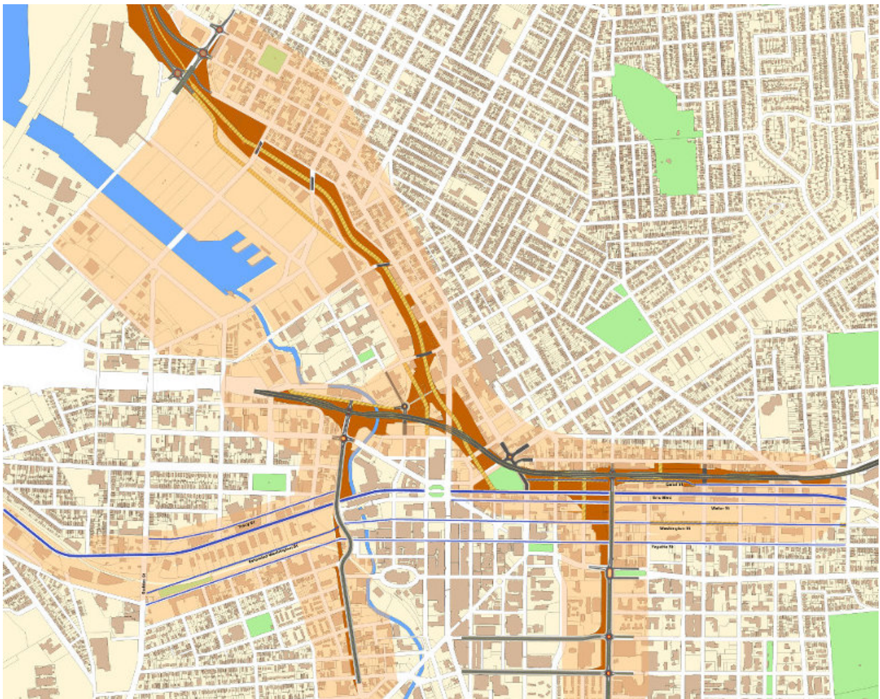
Figure 2: Full street-grid solution: newly available taxable and developable land (darker) plus nearby land of increased development interest (lighter). Yellow hashed lines represent new, fixed, or extended streets.
