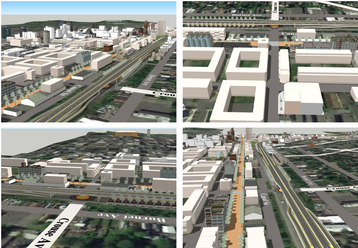
Figure 19: New I-690 half junction (easterly) at Crouse Ave (rough renderings); designed to coexist with Almond St full-junction; orange path is Erie Blvd as mixed-use residential/commercial pedestrian-friendly street; slimmed I-690 makes room to re-establish Canal St all the way to State St and provide rear access to a new row of buildings.
