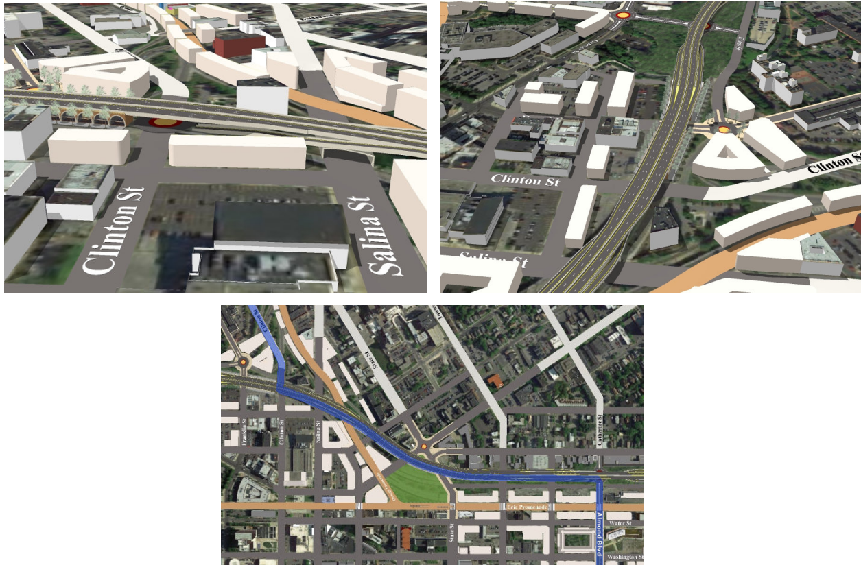
Figure 17: I-690 FCUI half-junction at Clinton St; provides a speedy and easily navigable north/south path (I-690 “land bridge” over downtown to Almond St); the required distance between Clinton St and West St ramps is achieved by foregoing unneeded westerly ramps.
