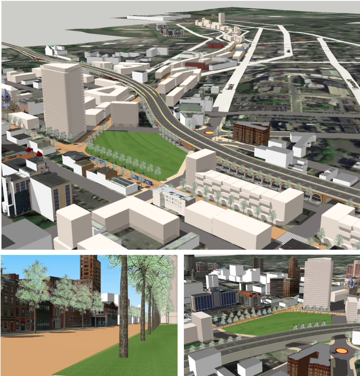
Figure 25: New Canalway Park (rough renderings): approximately 4 acres (in place of the downtown spaghetti junction); along “Erie Way”; I-690 is rebuilt as an archway viaduct with shops underneath. (Note: beige buildings represent new development.)
