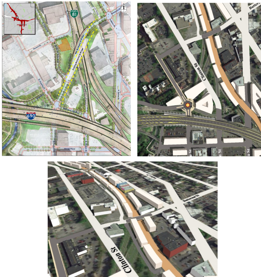
Figure 10: Butternut St Bridge: The CG proposal (left) keeps Webster’s Landing clogged with bridge and highway ramps. By building it straight across new and narrower “Oswego St” (right, bottom), Webster’s Landing is freed up for development.
