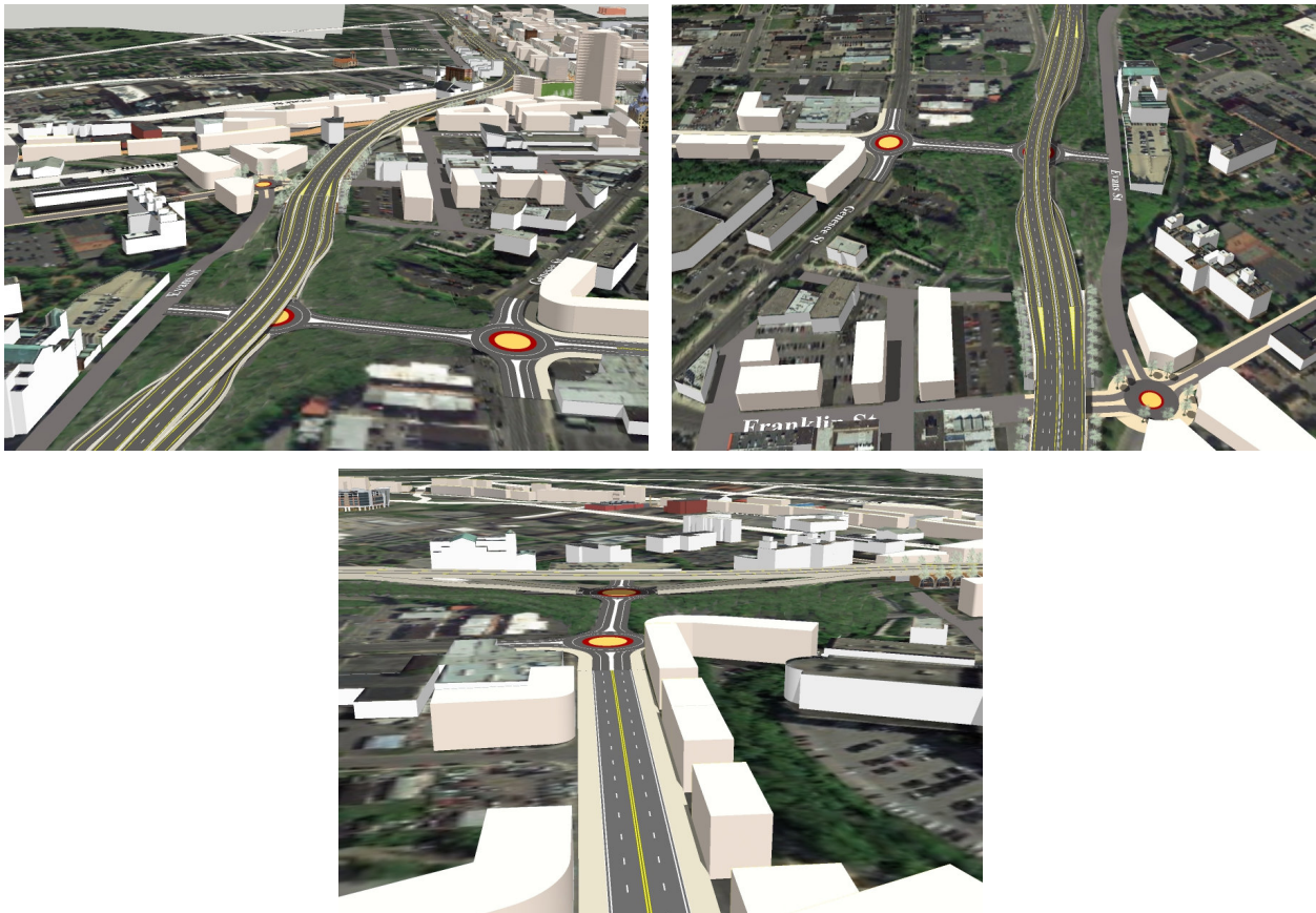
Figure 16: West St / I690 junction (rough renderings): redesigned as an FCUI to eliminate traffic light, significantly increase traffic flow rate, and provide easy connection to Evans St. A roundabout added at West St / Genesee St junction (below) further improves traffic flow.
