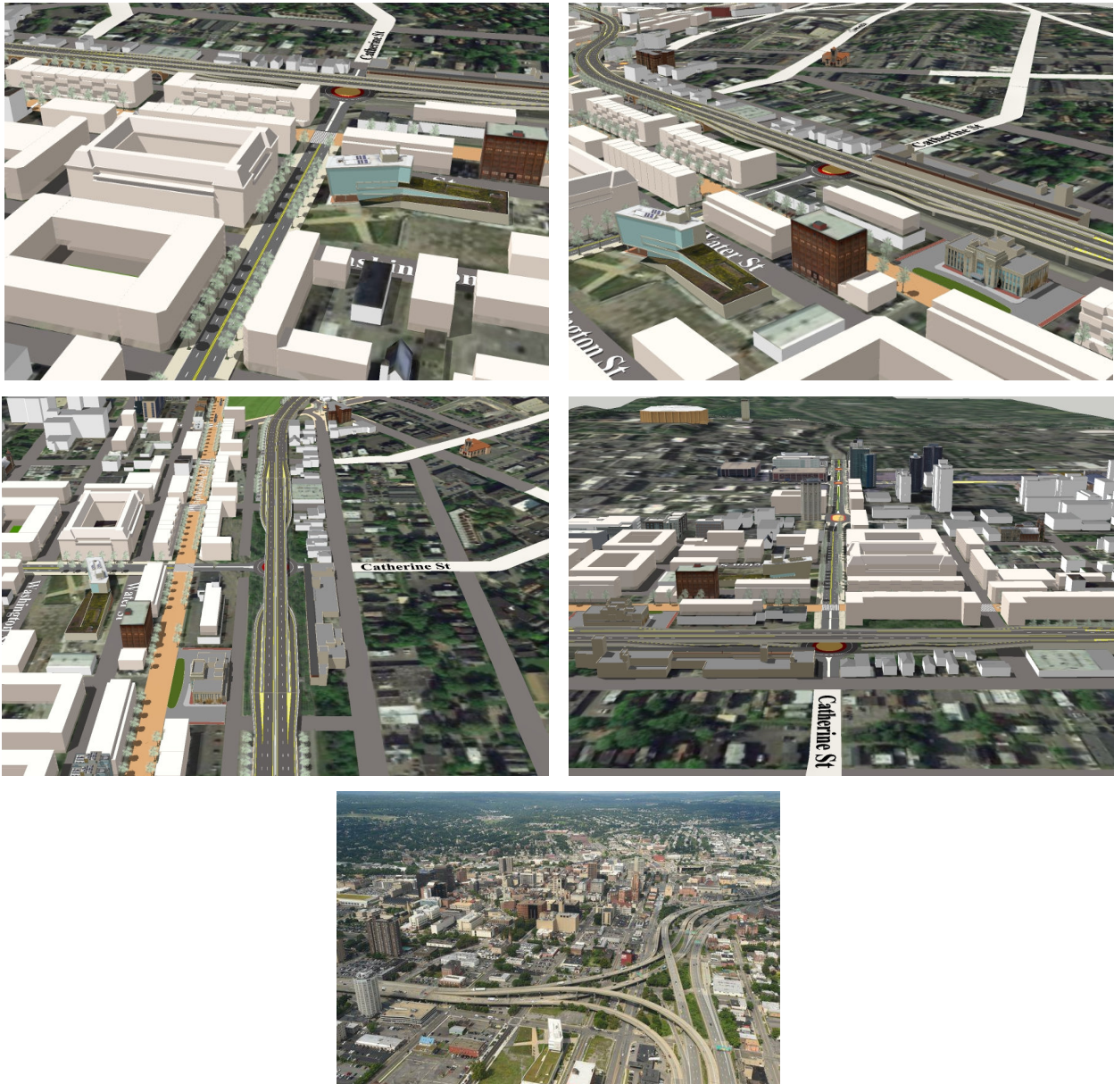
Figure 18: New Almond St / I690 junction; designed as an FCUI. The junction is crucial as part of a speedy and easily navigable north/south path through the city. Almond St area today (bottom).
