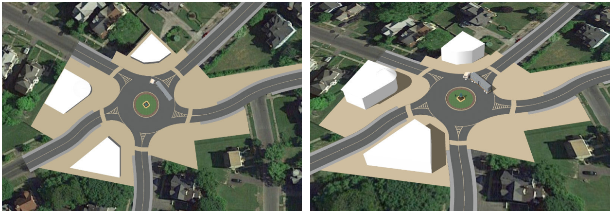
Figure 42: Onondaga Circle revived as a roundabout (top and angled view). Leftover ROW and adjacent private parcels form an attractive piazza-like environment, with new mid-rise, mixed-use buildings housing shops and restaurants, and apartments above. A new neighborhood gathering place.
